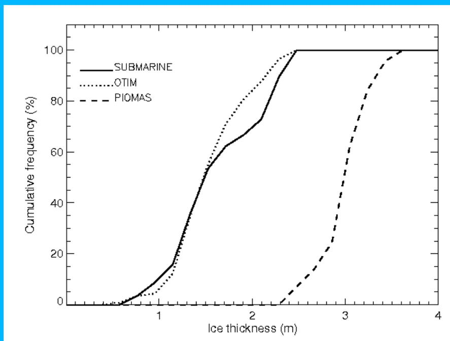
**Figure 9.** Comparisons of ice thickness cumulative distribution retrieved by OTIM with APP-x data, measured by submarine, and simulated by numerical model PIOMAS. Submarine ice draft (mean and median only) was already converted to ice thickness by a factor of 1.11.
