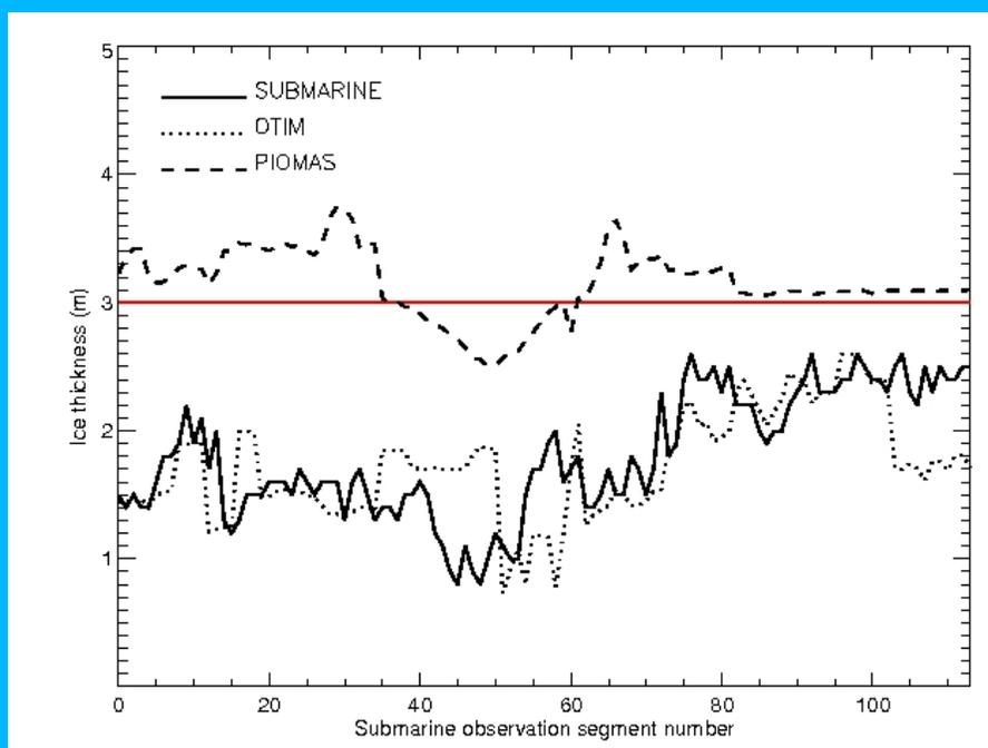
**Figure 10.** Comparisons of ice thickness values retrieved by OTIM with APP-x data, measured by submarine, and simulated by numerical model PIOMAS along the submarine track segments. Submarine ice draft (mean and median only) was already converted to ice thickness by a factor of 1.11.
