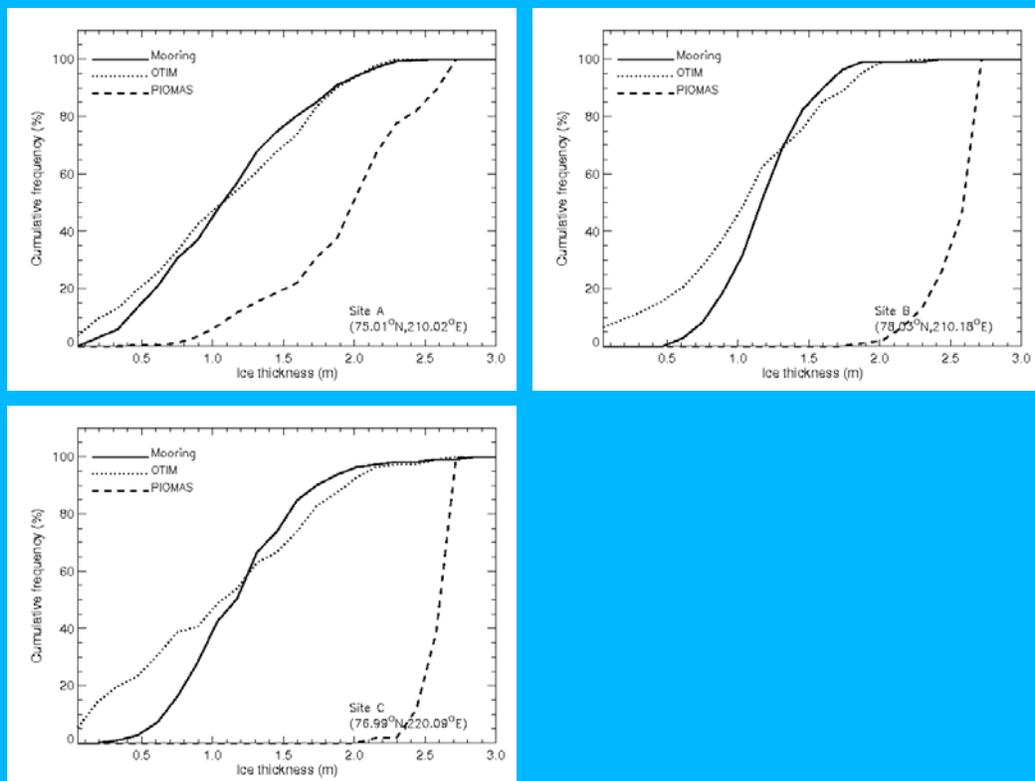
**Figure 14.** Comparisons of ice thickness cumulative distribution retrieved by OTIM with APP-x data, simulated ice thickness from the PIOMAS model and the ULS measurements at the mooring sites A, B, and C.
